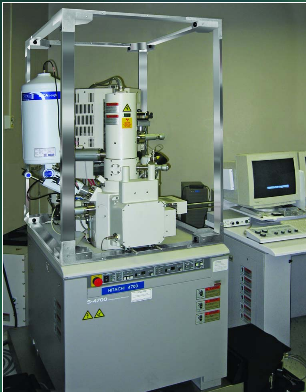
Mag-NetX™ System with Helmholtz coils mounted on a Hitachi S-4700 scanning electron microscope column console.
