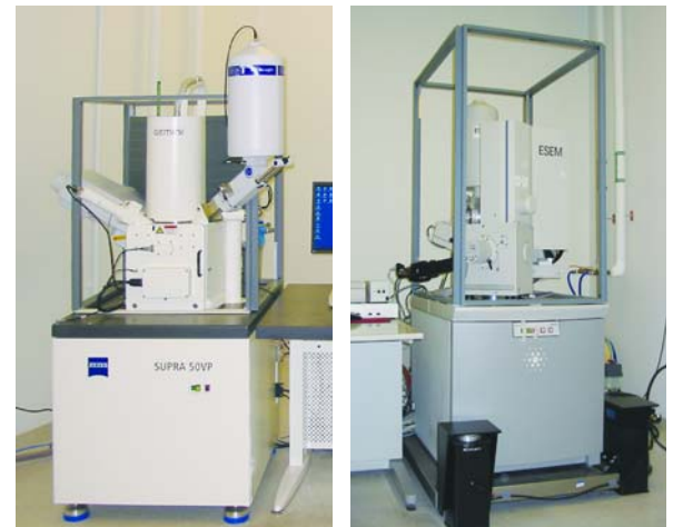
Photos courtesy of Drexel University. Mag-NetX™ Systems protect Zeiss Supra VP 50 (left) and FEI ESEM (right) scanning electron microscopes.
